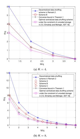
Fig. 2: The storage-load tradeoff for the decentralized data shuffling problem.
