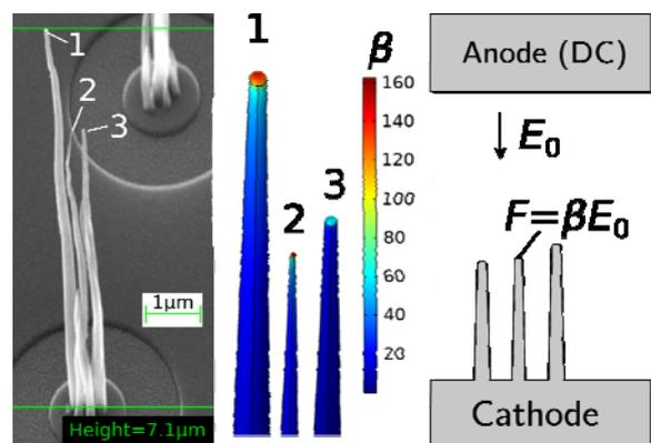
Fig. 1. Left: Electron beam microscope image of the studied bundle. Three carbon nanocones are identified and measured. Center: Colormap of the field enhancement factor  $\beta$  at the emitter surface. Right: scheme of the electrostatics simulation.
