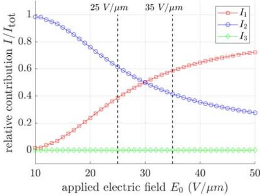
Fig. 2. Variation over the applied electric field of the emitter relative contribution to the total current of the bundle  $I_{\text{tot}}$
