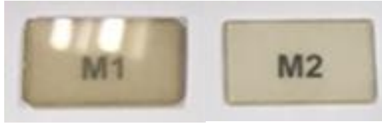
Figure 2: Optical photos of the optical ceramic samples: the thickness of M1 (left) is 1.032mm, the thickness of M2 (right) is 1.842mm
