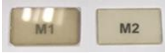
Figure 2: Optical photos of the optical ceramic samples: the thickness of M1 (left) is 1.032mm, the thickness of M2 (right) is 1.842mm
