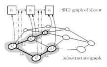
Fig. 3. Provisioning of infrastructure resource to an SRD graph: Resources from the infrastructure node  $i_1$  is provisioned for SRD node  $v_1$ ; Resources from  $i_2$  and  $i_4$  are provisioned for SRD node  $v_2$ ; and resources from  $i_3$  and  $i_5$  are provisioned for SRD node  $v_3$ . Correspondingly, the infrastructure links  $i_1i_2$  and  $i_1i_4$  are provisioned for SRD link  $v_1v_2$  and resources from links  $i_2i_3$  and  $i_4i_5$  are provisioned for SRD link  $v_2v_3$ .
