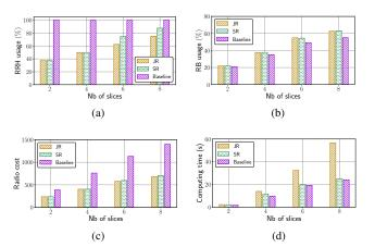
Fig. 5. Results of (a) utilization of RBs, (b) utilization of RRHs, (c) radio cost, and (d) computing time as a function of  $|\mathcal{S}|$ , with  $|\mathcal{N}_{Ir}| = 8$ .
