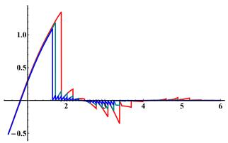
Fig. 1. Tracking Error  $\hat{x}_2(t)-x_2(t)$  Converging to 0 over Time with Sampling Rates  $\overline{T}$  (Red),  $0.5\overline{T}$  (Green), and  $0.25\overline{T}$  (Blue) with  $\overline{T}$  as defined in (51).
