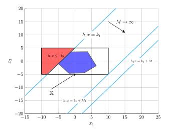
Figure 1: Illustration "big-M", M computed as in Remark 4. While the constraint is active (i.e.,  $\alpha_1=0$  in (9a)), the resulting inequality:  $-h_ix \leq -k_i$  describes the red region. Once  $\alpha_1=1$  (inactive/relaxed constraint), the selection of M gives the measure of relaxation. Thus, the idea is to relax sufficiently such that the remainder of the constraints is not affected.
