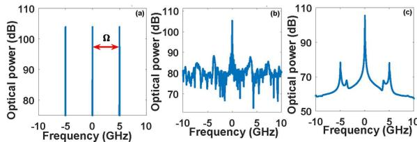
**Figure 1:** Optical spectra shown in (a) shows the injected comb for 3 comb lines, (b) free running injected laser and (c) injected laser under IL condition.  $\Omega = 5$  GHz is the comb spacing and  $\Delta\nu = 10$  MHz is the detuning.
