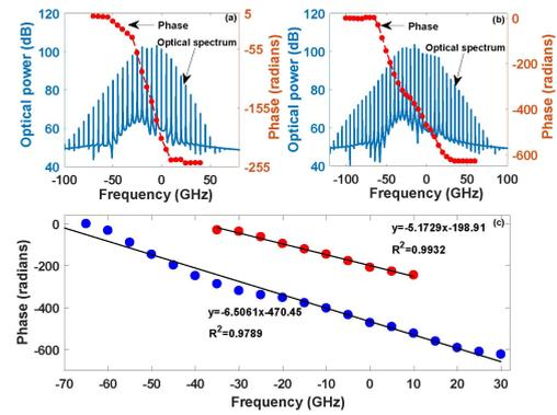
**Figure 5:** Optical spectra and phase for each comb line for  $\Delta\nu = 0$  GHz,  $\kappa = 0.8$  and  $\Omega = 5$  GHz. (a) and (b), optical spectra (left vertical axis), phase (right vertical axis) for 3 and 7 comb lines, respectively. (c) fitting of the linear part of the phase dependence for 3 comb lines (red) and 7 comb lines (blue)
