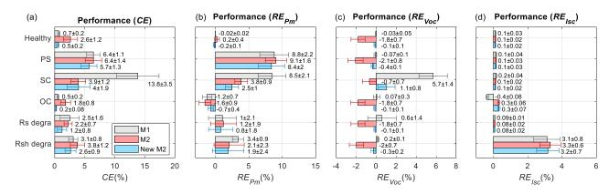
Fig. 4 Four metrics to present the correction performance of M1, M2 and NewM2: (a) *CE*, (b) *RE* of  $P_m$ , (c) *RE* of  $V_{oc}$ , (d) *RE* of *I<sub>SC</sub>* (the bars represent the mean value for the correction of 174 curves, while the horizontal whiskers represent the standard deviation (std), these 2 values are marked as 'mean'±'std')
