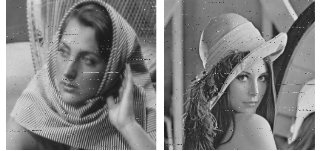
(c) Received image at node A, BER = 0.0128 (d) Received image at node B, BER = 0.0122
