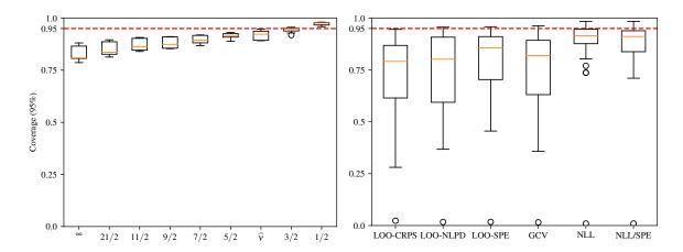
Figure 4: Box plots of  $C_{0.95}(\theta)$  (averaged over the repetitions for each test function). Left: for several regularities and using the NLL criterion on all 5d GKLS problems; right: for several selection criteria and for  $\nu$  automatically selected, on the whole set of test functions.
