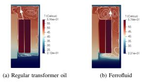
Fig. 2: Temperature field (°C) at t = 20000 s and velocity field streamlines. The arrow represents the flow direction.
