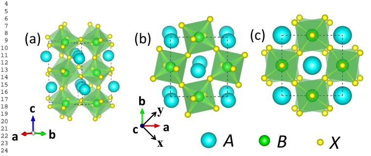
Figure 5: Panels (a) and (b) are sketches of the Pbmm perovskite  $ABX_3$ . Panel (a) is its three-dimensional view with the anti-phase tilting of  $BX_6$  shown along  $\mathbf{a} + \mathbf{b}$  direction; panel (b) is the top view with the in-phase tilting of  $BX_6$  along  $\mathbf{c}$  direction (also, z direction). Panel (c) sketches the I4/mcm perovskite  $ABX_3$ .
