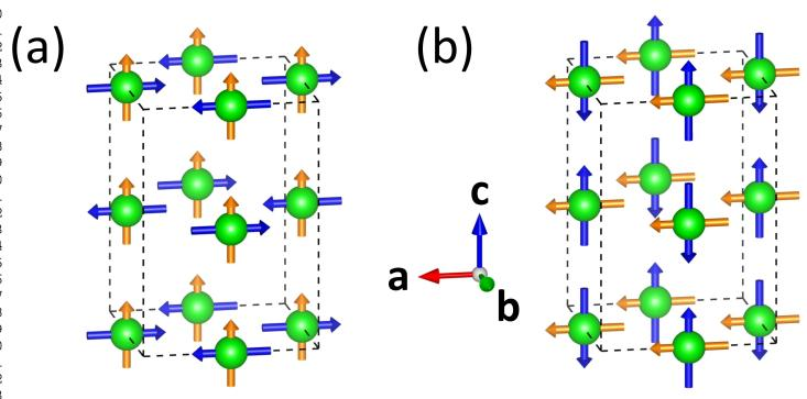
Figure 7: Two typical magnetic structures associated with the B-sublattice (green spheres) in  $ABX_3$  perovskites. The blue and yellow arrows denote the G-type antiferromagnetic components and weak ferromagnetic components, respectively. The lattice and Cartesian coordinate systems coincide with Figure 5.
