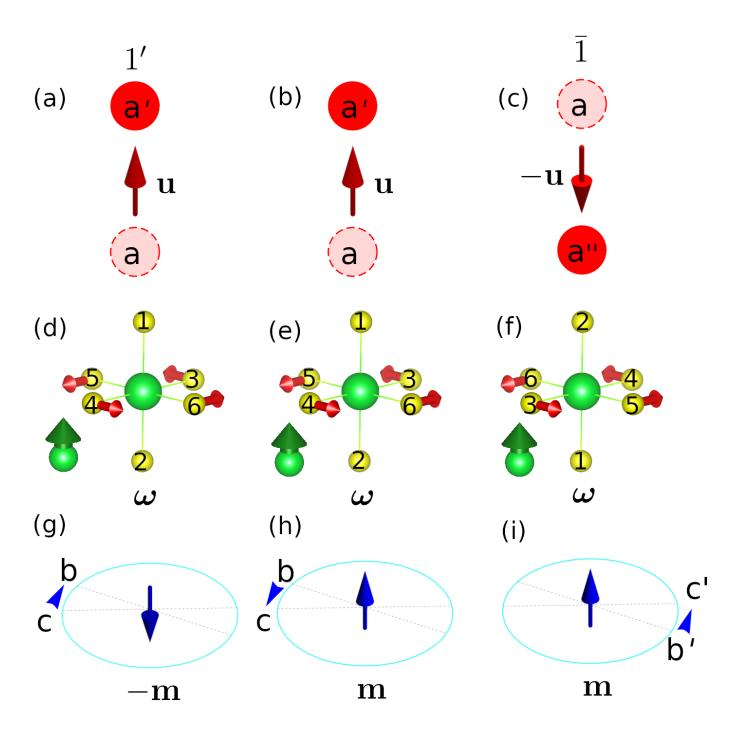
Figure 1: Sketches of displacement (b), rotation of  $BX_6$  octahedra (e) and magnetization (h) vectors, and their transformations under time reversal (a, d, g) and inversion (c, f, i). In panel b, the inversion center locates at the position bisecting "a" and "a'"; in panel e, the inversion is centered at the B ion (green sphere); in panel h, the inversion is the center of the cyan circle.
