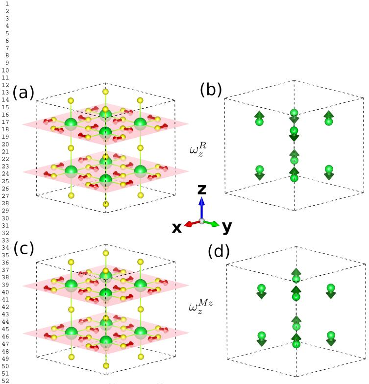
Figure 2: Sketches of anti-phase (a) and in-phase (c) tiltings of  $BX_6$  octahedra about the z direction for  $ABX_3$  perovskites, and their representations by the  $\omega$  vectors (b, d). Here, the green and yellow spheres denote the B and X ions, while the A ions are not shown for clarity.
