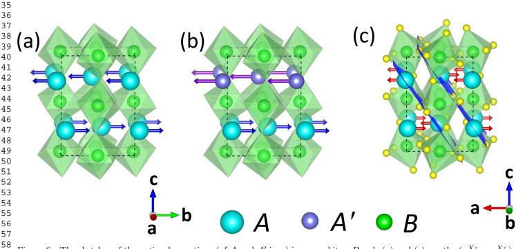
Figure 6: The sketches of the anti-polar motions (of A and A' ions) in perovskites. Panels (a) and (c) are the  $(u_{A,x}^{Xz}, -u_{A,y}^{Xz})$ , and  $(u_{A,x}^R, u_{A,y}^R)$  motions of  $Pbnm\ ABX_3$  perovskite, respectively. Panel (b) shows the displacement mode for  $ABX_3/A'BX_3$  superlattice. The lattice and Cartesian coordinate systems coincide with Figure 5.
