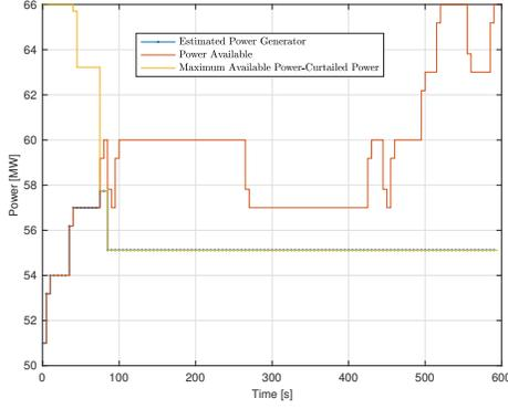
Fig. 4. The power variables in the power generator at node 2076 from the MPC result with prediction horizon  $N=10$ . The yellow one depicts  $\bar{P}_n^G - P_n^C(k)$ , the red line represents  $P_n^A(k)$ , and the dotted blue one is  $P_n^G(k)$ .
