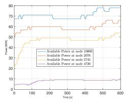
Fig. 2. The available powers for the four generators.
