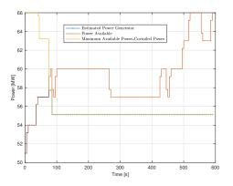
Fig. 4. The power variables in the power generator at node 2076 from the MPC result with prediction horizon N=10. The yellow one depicts  $\overline{P}_n^C - P_n^C(k)$ , the red line represents  $P_n^A(k)$ , and the dotted blue one is  $P_n^G(k)$ .
