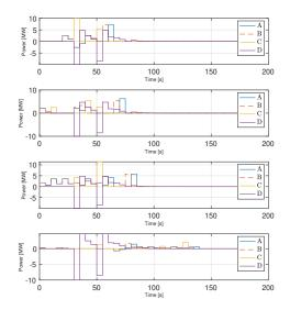
Fig. 7.  $\Delta P_n^G$  at the generators 10000, 2076, 2745, and 4720. The prediction horizon is N=10. A) Real  $\Delta P_n^G$ ; B) Estimated  $\Delta P_n^G$ ; C) Curtailment action; D) Battery action.
