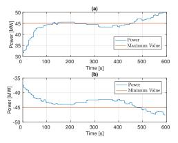
Fig. 3. The power flow on the branches in the open-loop simulation. (a): between buses 2745 and 1445. (b): between buses 2135 and 2076.
