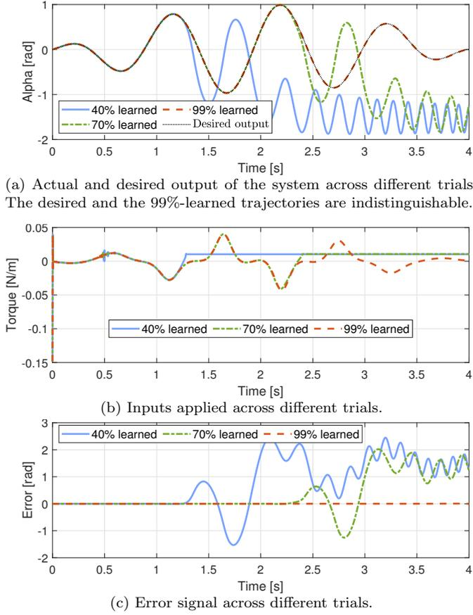
Fig. 3. Simulation results for desired trajectory #2.
