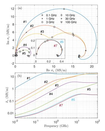
FIGURE 7: Multi-layer coating: (a) apparent conductivity and (b) dissipative apparent conductivity, for the seven coatings structures described in Table 2 and a thickness  $w_c=10~\mu\mathrm{m}$ .
