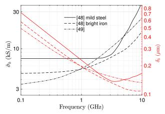
FIGURE 4: Power dissipation in bulk steel: effective dissipative conductivity  $\tilde{\sigma}_b$  and skin depth  $\delta_b$  versus frequency, for a DC conductivity  $\sigma_b = 6$  MS/m.
