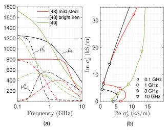
FIGURE 3: Bulk steel: (a) complex permeability  $\mu_b = \mu_b' - \mathrm{j}\mu_b''$  and effective dissipative permeability  $\tilde{\mu}_b$ , defined in (7); (b) effective bulk conductivity  $\sigma_b'$ , based on a conductivity  $\sigma_b = 6$  MS/m. Results processed from steel magnetic permeability data reported in the references in the legend.
