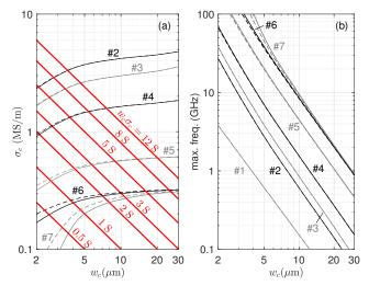
FIGURE 10: Equivalent single-layer modelling of multilayered coatings: (a) equivalent conductivity  $\sigma_c$  versus coating thickness, for structures #2 to #7 described in Table 2, for a  $\Gamma$  layer conductivity equal to 7 kS/m (solid curves) and 70 kS/m (dashed curves); red lines show the loci of constant  $w_c\sigma_c$  products. (b) maximum frequency for the transient region versus coating thickness.
