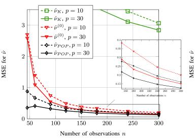
Fig. 1: Mean Square Errors of  $\hat{\nu}$  versus the number n of observations by running the different algorithms until convergence (MAX 5 iterations), using initial value  $\nu_0$ . The samples are generated from a p-variate real  $t_3(\mathbf{0}, \mathbf{\Sigma})$ -distribution, where  $\mathbf{\Sigma}$  has an AR(1) covariance matrix structure with  $\varrho=0.6$  and p=10 (dashed curves) and 30 (plain curves); 5000 Monte Carlo runs.
