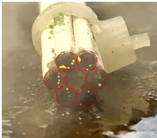
Fig. 7: third step of crackle: appearance of luminous points on the surface of the anode core and degradation of the anode.
