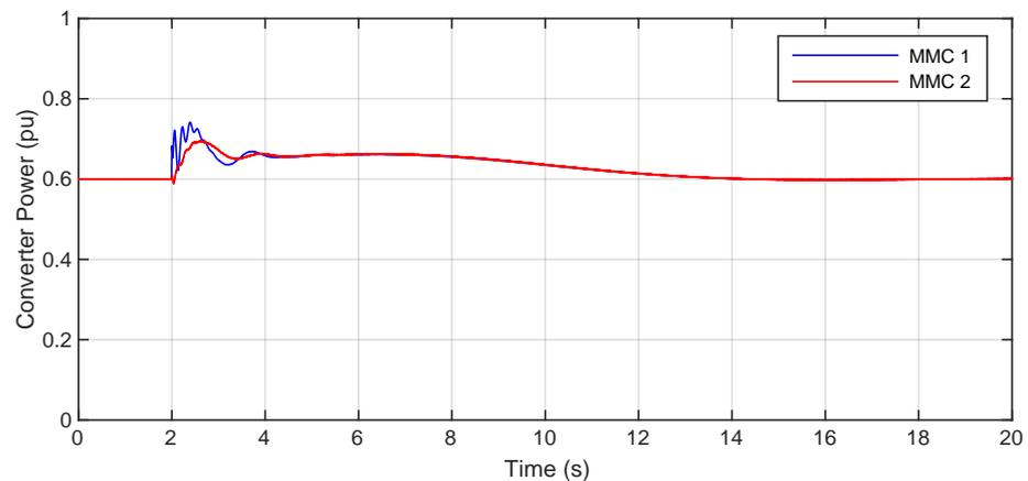
**Figure 13.** Power injected by the HVDC converter terminals after the disturbance in Scenario 2.
