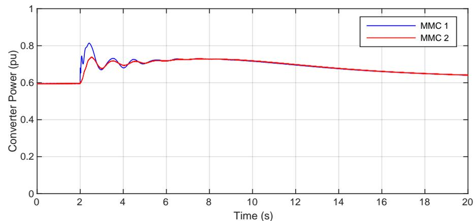
**Figure 10.** Power injected by the HVDC converter terminals after the disturbance in Scenario 1.
