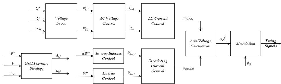
**Figure 4.** Block diagram of an MMC-based GFM converter.
