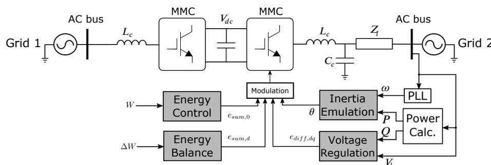
Figure 5. VSM general control scheme applied to an MMC-HVDC link.
