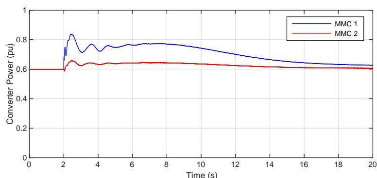
**Figure 16.** Power injected by the HVDC converter terminals after the disturbance in Scenario 3.
