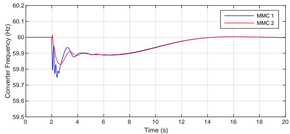
**Figure 12.** Frequency of the voltage generated at the HVDC converter terminals after the disturbance in Scenario 2.
