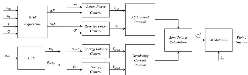
**Figure 3.** Block diagram of an MMC-based GFL converter embedded with supporting capabilities.
