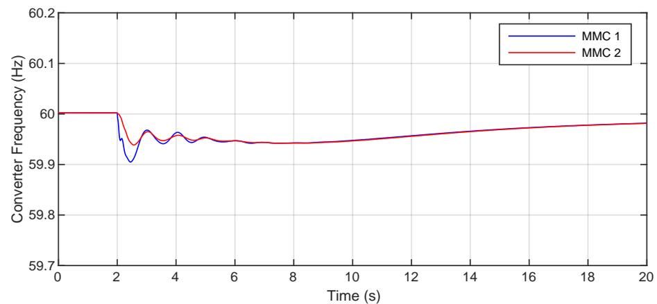
**Figure 9.** Frequency of the voltage generated at the HVDC converter terminals after the disturbance in Scenario 1.
