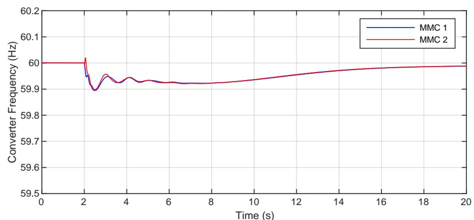
**Figure 15.** Frequency of the voltage generated at the HVDC converter terminals after the disturbance in Scenario 3.
