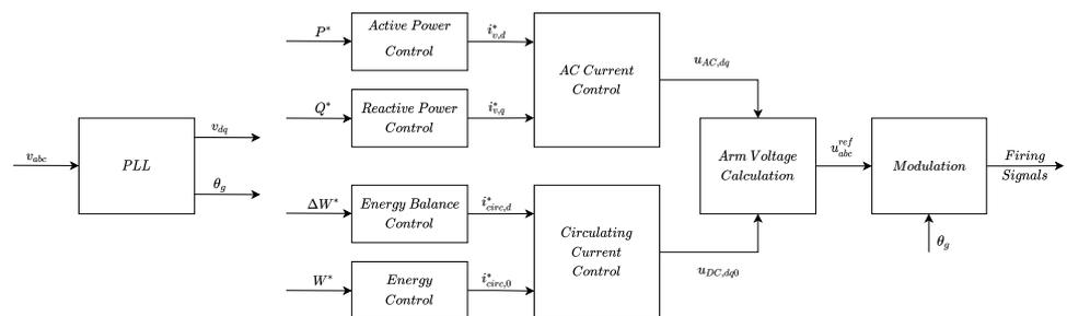
Figure 2. Block diagram of an MMC-based GFL converter in grid-feeding mode.
