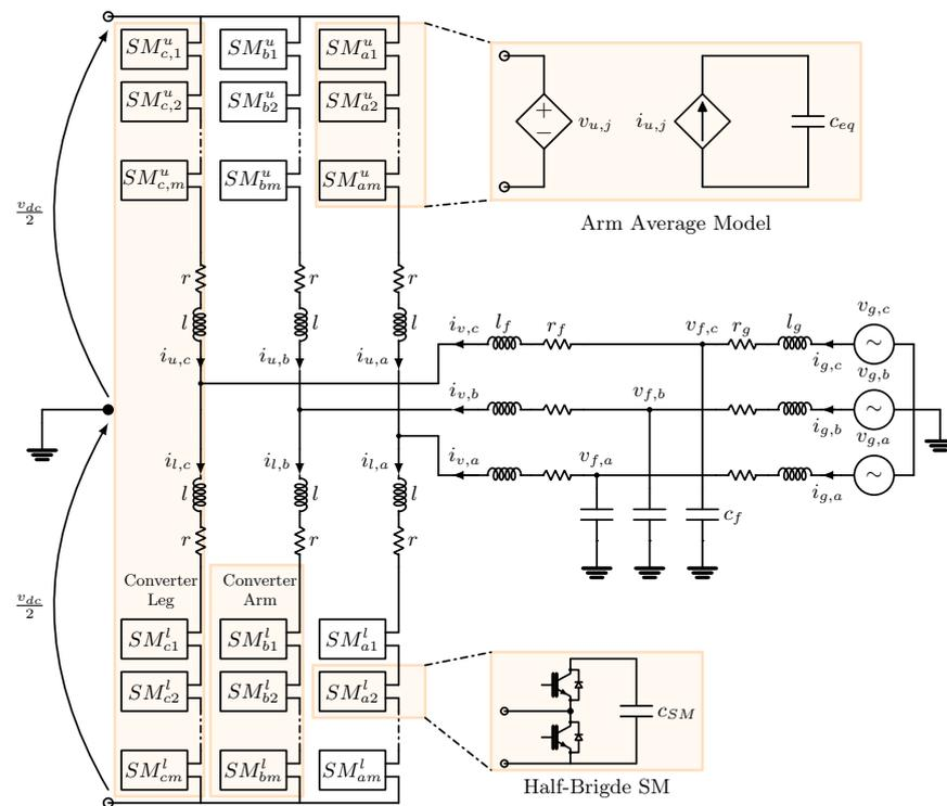
Figure 1. Model of an MMC-HVDC inverter terminal connected to the electric grid.
