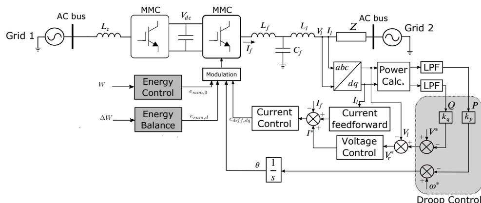
Figure 6. Droop general control scheme applied to an MMC-HVDC link.
