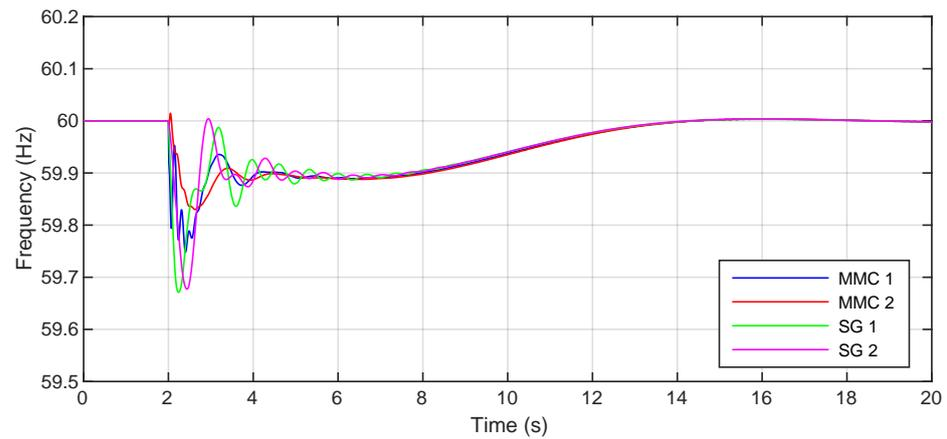
**Figure 11.** Frequency behavior of the elements of the test system after disturbance in Scenario 2.
