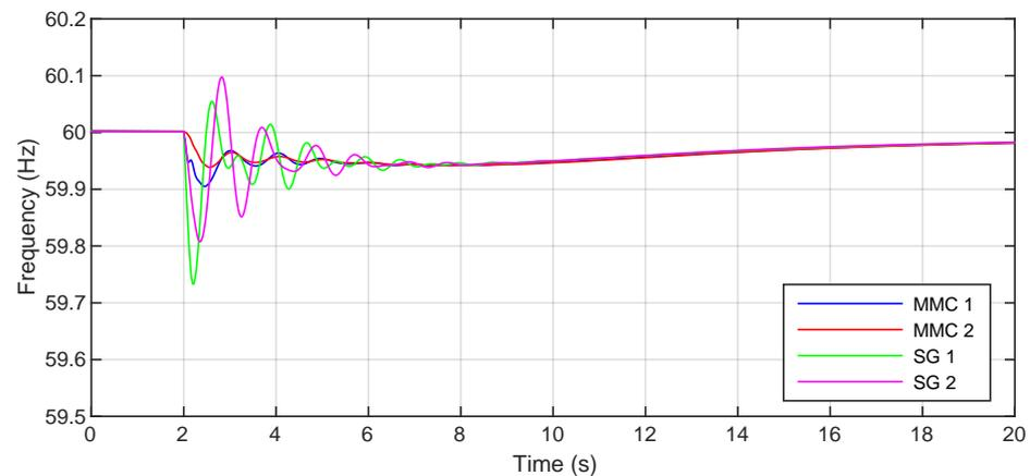
**Figure 8.** Frequency behavior of the elements of the test system after disturbance in Scenario 1.
