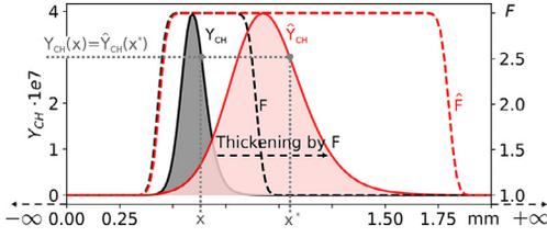
Fig. 1. Impact of the flame thickening by intermediate species (CH) mass fraction with  $F_{\max} = 3$ . Black lines: non-thickened quantities  $\varphi$ . Red line: thickened quantities  $\hat{\varphi}$ . Thickening increases the total amount of the species (illustrated by the gray area) to a much greater amount (illustrated by the transparent red area). (For interpretation of the references to color in this figure legend, the reader is referred to the web version of this article.)
