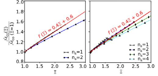
Fig. 4. Normalized mass of CO in term of subgrid-scale flame wrinkling  $\Xi$  at a filter size  $\Delta = 5\delta_l^0$  (left) and  $\Delta = 10\delta_l^0$  (right), where  $\delta_l^0$  is the laminar flame thickness. Results are plotted for different numbers of flame patterns  $n_\Delta$ . Extracted from [14].
