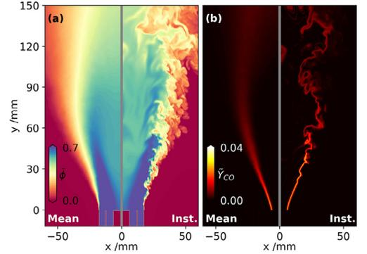
Fig. 5. Mean (left sub-figure) and instantaneous (right sub-figure) equivalence ratio  $\phi$  (a) and CO mass fraction  $\hat{Y}_{CO}$  (b) in a section through the centre-line.
