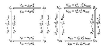
FIG. 1. Relations among the four piezoelectric (left) and electrostrictive (right) tensors, via the elastic constant  $(c_{ijkl})$  and compliance  $(s_{ijkl})$  tensors, the electric susceptibility tensor  $(\varepsilon_0\chi_{ij})$ , and its inverse  $(\eta_{ij})$  in linear dielectric and elastic materials under isothermal or isentropic conditions. Exponents refer to the variables held constant.
