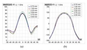
Fig. 5. (a) Magnitude and (b) phase of the differential transmission coefficient computed for various maximum deviations as a function of the stroke position.
