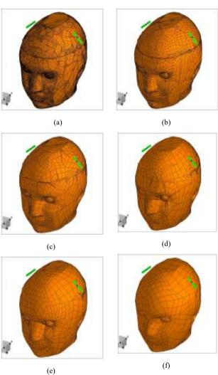
Fig. 2. The outer surface of the numerical phantom represented by a quadrilateral mesh with (a)  $\sigma_{max} = 0.00$  mm, (b)  $\sigma_{max} = 0.75$  mm, (c)  $\sigma_{max} = 1.50$  mm, (d)  $\sigma_{max} = 2.25$  mm, (e)  $\sigma_{max} = 3.00$  mm, and (f)  $\sigma_{max} = 4.50$  mm.
