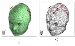
Fig. 3. The inner sufaces of the numerical phantom represented by a quadrilateral mesh (a) homogeneous brain, (b) stroke at three different locations ( $\sigma_{max} = 3$  mm).
