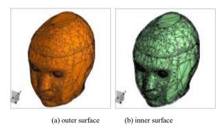
Fig. 1. The numerical phantom is represented by a triangular mesh.
