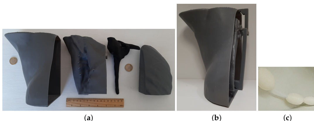
Figure 8. Three-dimensional-printed phantom. (a) From left to right: (i) torso, (ii) muscle, (iii) bone, and (iv) lung cavities, together with the (iii) bone structure are represented. (b) Assembled phantom, where we can observe an extra part which keeps the organs in place inside the other container. (c) Three ellipsoidal hollow axillary lymph nodes, with a wire passing through them.
