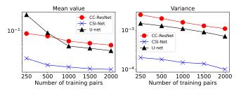
Fig. 7. Mean and variance of  $\mathrm{Err}_\chi$  obtained by CC-ResNet, CSI-Net and U-net on 200 test samples as a function of the number of training pairs.
