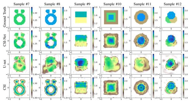
Fig. 9. Reconstructed relative permittivity obtained by CSI-Net, U-net, and CSI. The models are trained with the circular dataset. The test dataset lies outside the range of training data. 20 dB Gaussian noise affects the collected scattered fields.
