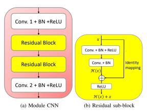
Fig. 2. Network structure of Module CNN and its residual sub-block.
