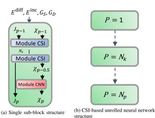
Fig. 1. CSI-based unrolled neural network structure.  $p \in \{1 \dots N_p\}, N_p$  number of sub-blocks.  $k \in \{1 \dots N_k\}, N_k$  number of CSI iterations in each.
