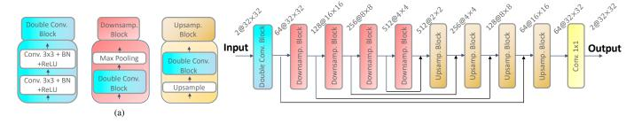
Fig. 3. The U-net structure. The dimension of the feature maps passing through each layer is noted as [Number of channels@ $H \times M$ ].
