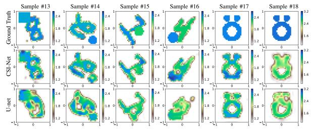
Fig. 10. Reconstructed relative permittivity obtained by CSI-Net, U-net (CSI has been omitted since failing to yield proper reconstruction). The models are trained with the MNIST dataset. The test dataset is outside the range of training data. 20 dB Gaussian noise affects the collected scattered fields.
