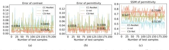
Fig. 5.  $\text{Err}_{\chi}$ ,  $\text{Err}_{\varepsilon}$  and SSIM obtained by applying the trained model on 200 test samples. Gaussian noise of SNR = 20 dB is added to collected fields.
