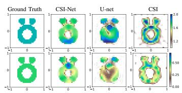
Fig. 11. Reconstructed relative permittivity obtained by models trained with a complex-valued circular dataset.  $\Re\{\varepsilon\}$  (top) of ground truth is 1.8 and  $\Im\{\varepsilon\}$  (bottom) is 0.5. 20 dB Gaussian noise affects the collected scattered fields.
