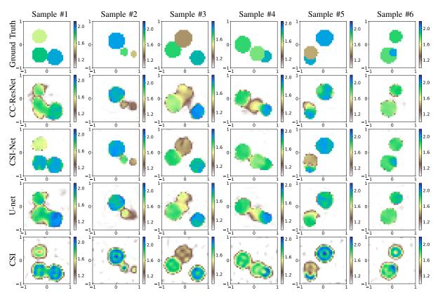
Fig. 4. Relative permittivity of reconstructed profiles from the test dataset. The range of relative permittivity is [1.3, 2]. Gaussian noise of SNR =  $20 \, \mathrm{dB}$  is added. The first row is the ground truth of the profiles.
