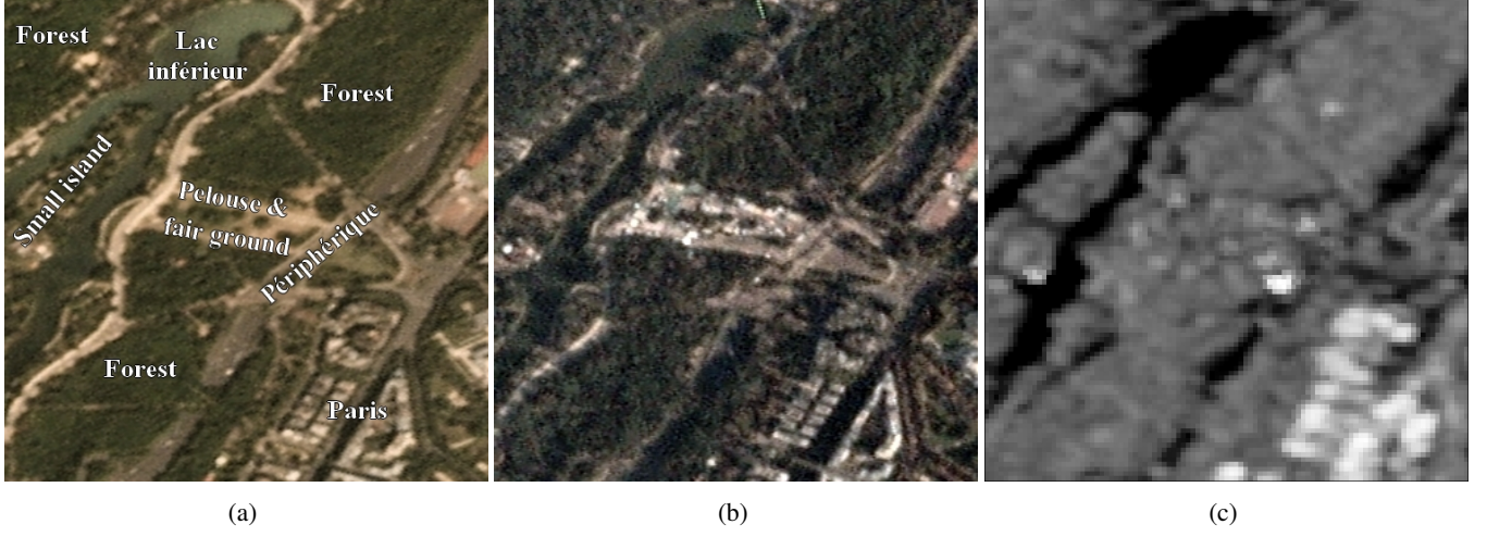
Fig. 2: Parts of the Bois de Boulogne : (a) annotated optical image without the fair (2020/04/24, © Planet Labs PBC [11]), (b) optical image with the fair (2020/09/13, © Planet Labs PBC [11]), (c) temporal mean of SAR images (Ascending VV, 30 dates).
