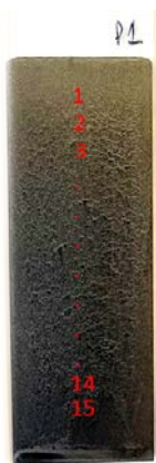
Fig.12: Charged sol-gel coating deposited on glass at constant speed showing the locations of R_s measurements.
