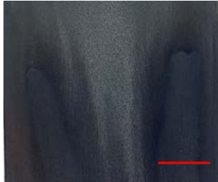
Fig.7: Example of clear and dark zones observed on sol-gel [A] coatings; red scale:10mm.
