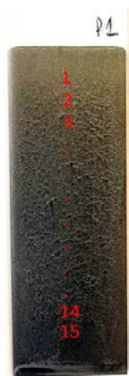
Fig.12: Charged sol-gel coating deposited on glass at constant speed showing the locations of R_s measurements.
