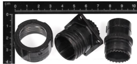
Fig.4: Connector housing coated with the charged sol-gel process [8]
