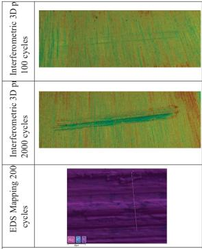
Table 2: 3D interferometric profiles and SEM/EDS elemental mapping of AgC worn surfaces, under 400 MPa
