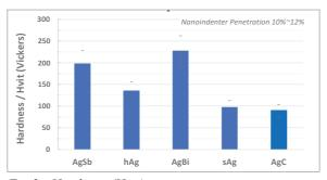
Fig.2: Hardness (Hvit) measurements, using nanoindentation, on flats electroplated with various silver based deposits
