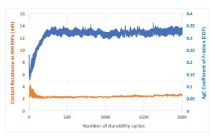
Fig.4.1: Electrical Contact Resistance and Friction Coefficient evolution of AgC silver-carbon electrodeposit according to durability cycles
