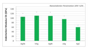
Fig.3: Indentation modulus measurements, using nanoindentation, of flats electroplated with various silver based deposits
