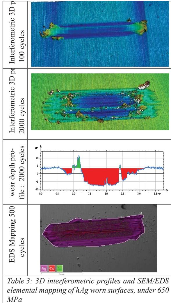
Table 3: 3D interferometric profiles and SEM/EDS elemental mapping of hAg worn surfaces, under 650 MPa
