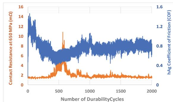
Fig.4.2 : Electrical Contact Resistance and Friction Coefficient evolution of hAg Hard Pure Silver electrodeposit according to durability cycles
