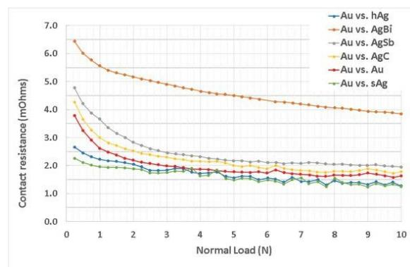
Fig.1 : Contact resistance evolution vs. normal force between between Au/Ni hemispheres & flats plated
