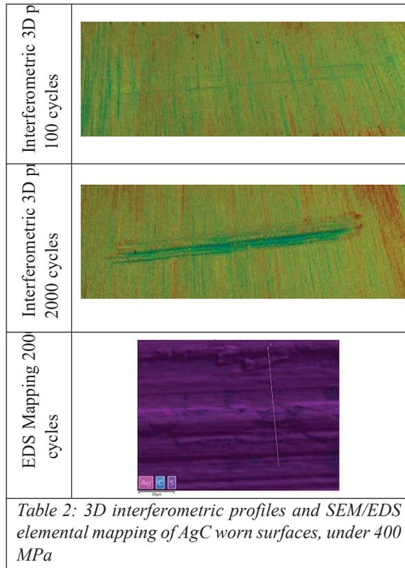
Table 2: 3D interferometric profiles and SEM/EDS elemental mapping of AgC worn surfaces, under 400 MPa
