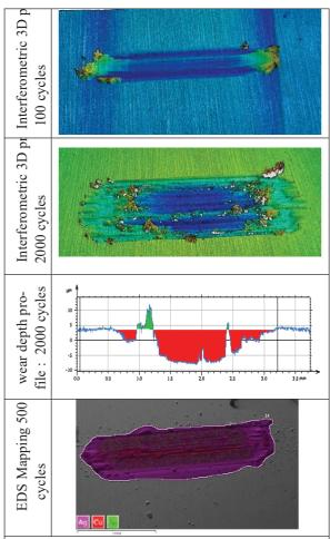
*Table 3: 3D interferometric profiles and SEM/EDS elemental mapping of hAg worn surfaces, under 650 MPa*
