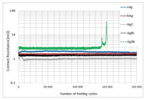
Fig.4.3 : Electrical Contact Resistance evolution of various silver-based deposits according to the number of fretting cycles under 650 MPa of contact pressure
