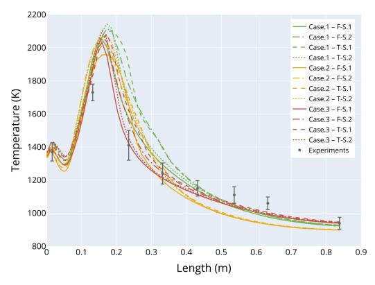
**Figure 4.** The evolution of the flame's temperature along the axis of the reactor for the different cases. Experimental data by [29].
