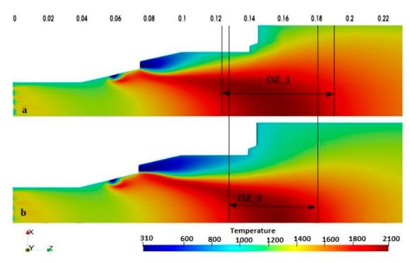
**Figure 3.** Temperature 2D surface plot in the entire reactor when adopting the same chemical kinetic mechanism F-S.1 for: (a)—Case 1 and (b)—Case 3.
