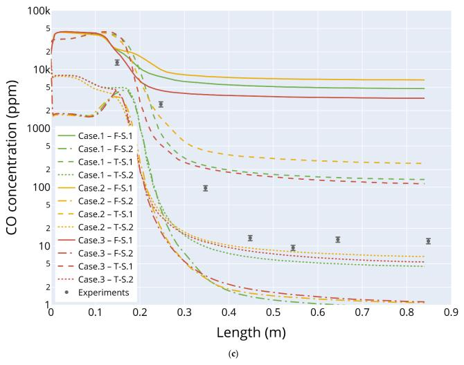
**Figure 5.** (a) The CO<sub>2</sub> volume fraction evolution along the center-line of the reactor. Experimental data by [29]; (b) The O<sub>2</sub> mole fraction evolution along the center-line of the reactor. Experimental data by [29]; (c) The CO concentration evolution along the center-line of the reactor. Experimental data by [29].
