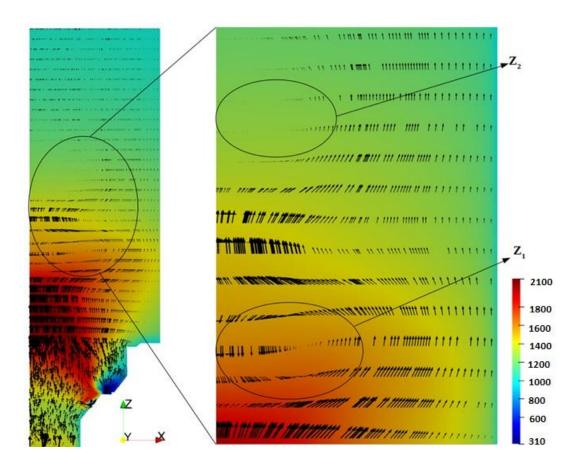
**Figure 6.** Velocity field and temperature contours for case 1 when adopting the chemical mechanism T-S.1.
