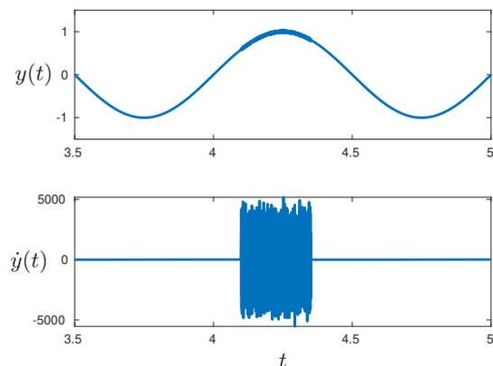
Fig. 1. Derivative effect on signal with small noise.
