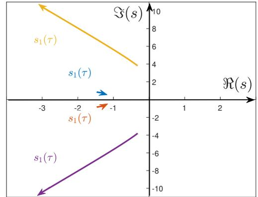
Fig. 7. Roots behavior of properly-posed system (18).
