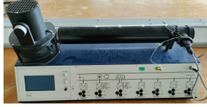
FIG. 1: Instrumented heat blower. The actuators (blower fan and heating resistance) are situated on the left of the picture, while the flow meter and thermocouple are on the right.
