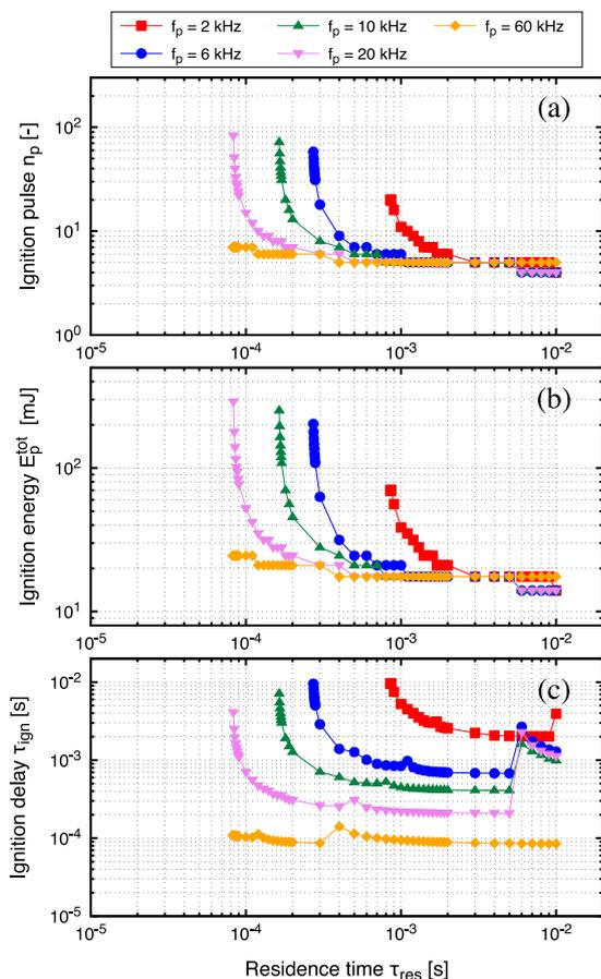
Fig. 10. Plasma-assisted ignition diagrams. (a) Number of pulses  $n_p$ , (b) total deposited energy  $E_p^{tot}$ , and (c) ignition delay time  $\tau_{ign}$  required to ignite the methane-air mixture ( $\phi = 0.95$ ) in terms of the residence time  $\tau_{res}$  for various pulse repetition frequency  $f_p$ . The pulse energy is fixed at  $E_p = 3.5$  mJ.
