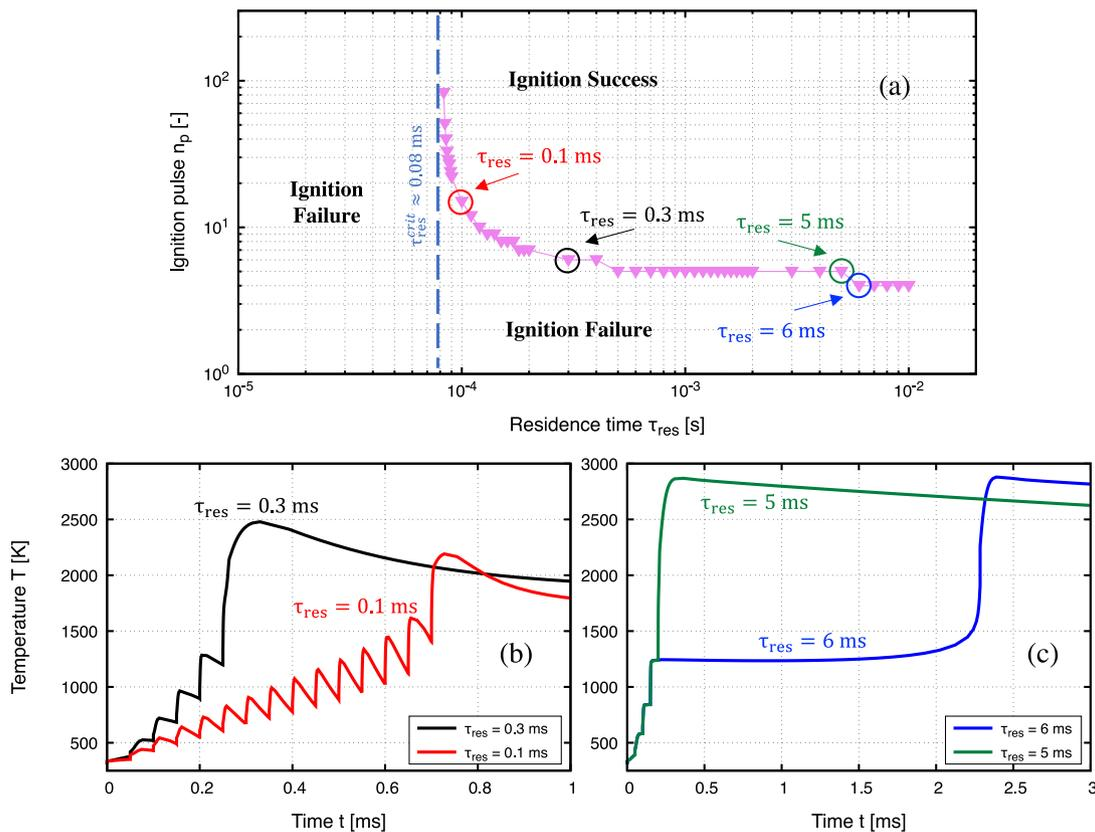
Fig. 5. (a) Minimum number of pulses  $n_p$  required to ignite the methane-air mixture ( $\phi = 0.95$ ) as a function of the residence time  $\tau_{res}$ . Temporal evolution of temperature (b) for two residence times of  $\tau_{res} = 0.1$  and  $0.3$  ms, and (c) for two residence times of  $\tau_{res} = 5$  and  $6$  ms. The pulse energy and the pulse repetition frequency are, respectively, fixed at  $E_p = 3.5$  mJ and  $f_p = 20$  kHz.
