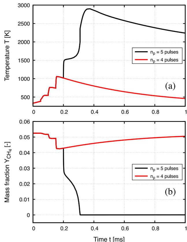
Fig. 4. Typical temporal profiles of (a) temperature and (b) methane mass fraction for  $f_p = 20$  kHz,  $E_p = 3.5$  mJ, and  $\tau_{res} = 0.5$  ms. Black profiles are obtained by applying five discharge pulses and red profiles by four discharge pulses. (For interpretation of the references to color in this figure legend, the reader is referred to the web version of this article.)
