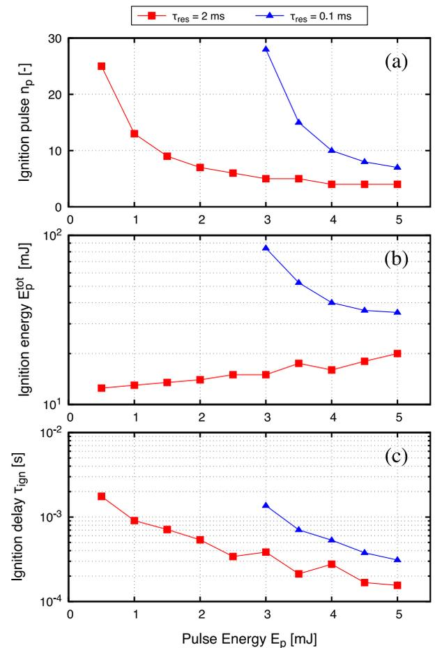
Fig. 8. Effect of pulse energy  $E_p$  on (a) number of pulses  $n_p$ , (b) total deposited energy  $E_p^{tot}$ , and (c) ignition delay  $\tau_{ign}$  for two residence times  $\tau_{res} = 0.1$  and 2 ms.  $f_p = 20$  kHz. The pulse repetition frequency is fixed at  $f_p = 20$  kHz.
