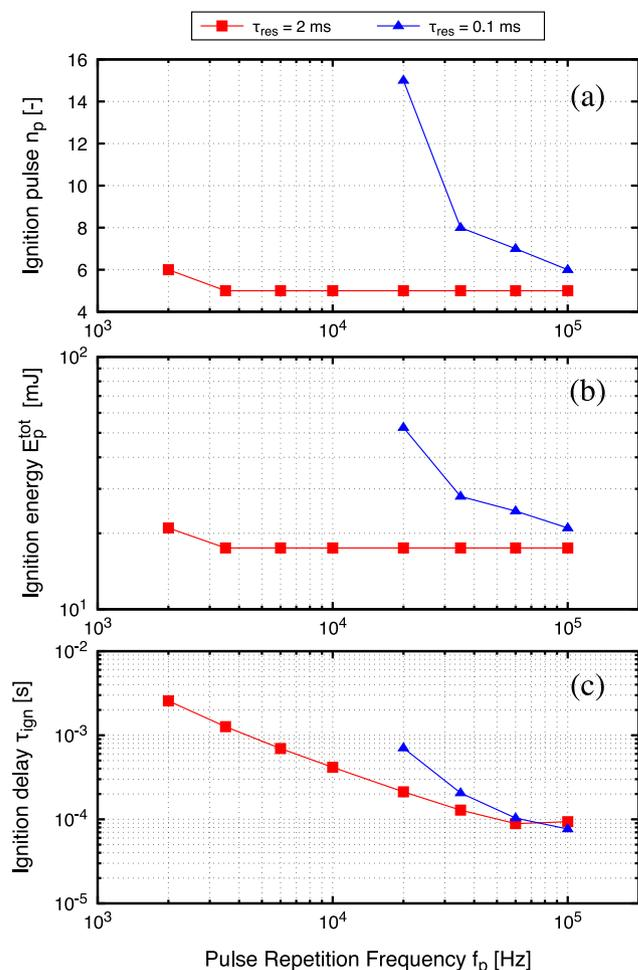
Fig. 11. Effect of pulse frequency  $f_p$  on (a) number of pulses  $n_p$ , (b) total deposited energy  $E_p^{tot}$ , and (c) ignition delay  $\tau_{ign}$  for two residence times  $\tau_{res} = 0.1$  and 2 ms. The pulse energy is fixed at  $E_p = 3.5$  mJ.
