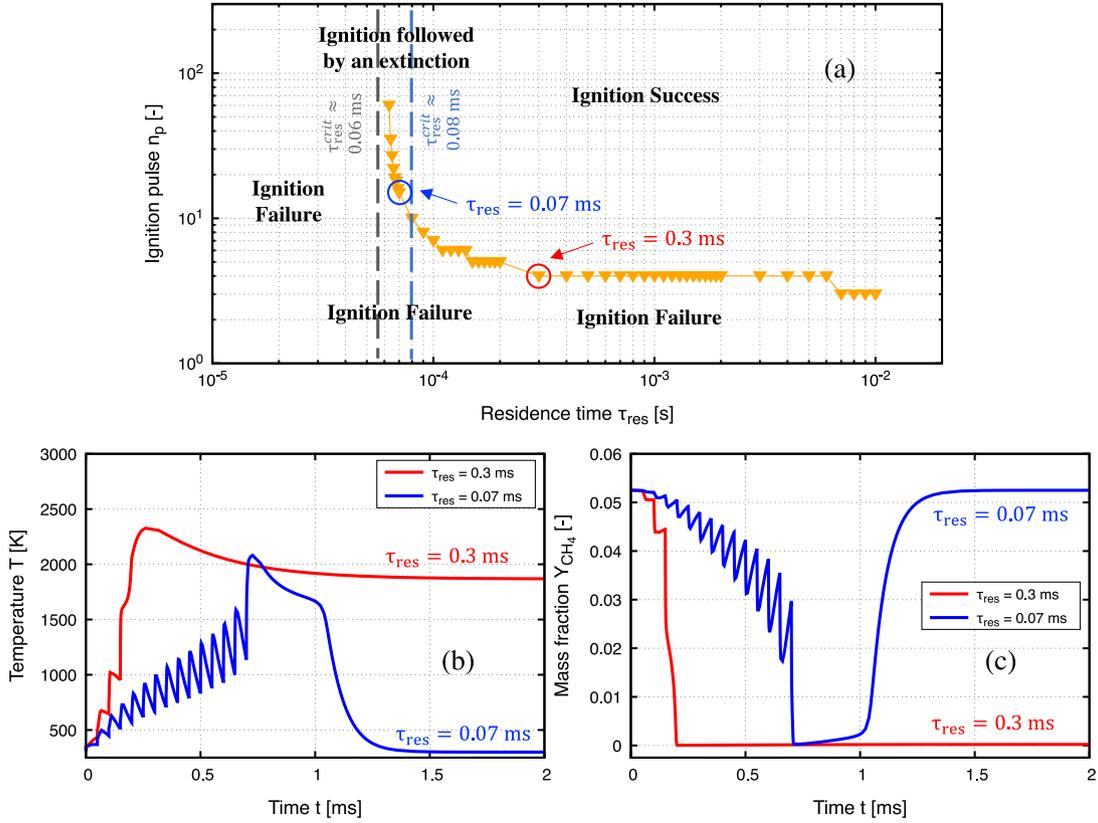
Fig. 6. (a) Minimum number of pulses  $n_p$  required to ignite the methane-air mixture ( $\phi = 0.95$ ) as a function of the residence time  $\tau_{res}$  for a pulse energy of  $E_p = 5.0$  mJ and a pulse repetition frequency of  $f_p = 20$  kHz. Temporal evolution of (b) temperature and (c) methane mass fraction for two residence times of  $\tau_{res} = 0.07$  and  $0.3$  ms.
