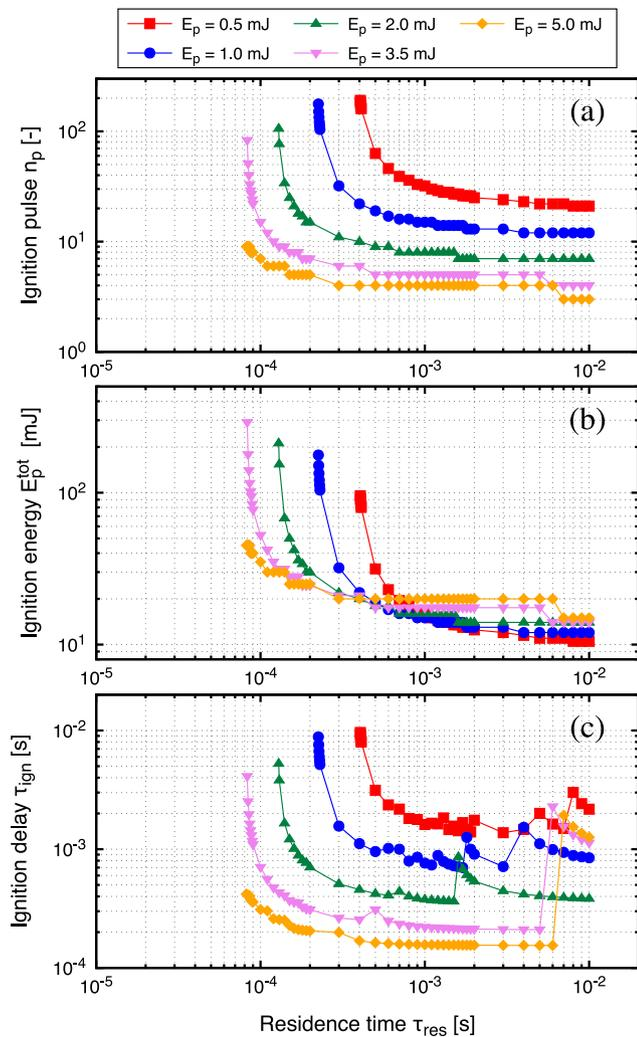
Fig. 7. Plasma-assisted ignition diagrams. (a) Number of pulses  $n_p$ , (b) total deposited energy  $E_p^{tot}$ , and (c) ignition delay time  $\tau_{ign}$  required to ignite the methane-air mixture ( $\phi = 0.95$ ) in terms of the residence time  $\tau_{res}$  for various pulse energy  $E_p$ . The pulse repetition frequency is fixed at  $f_p = 20$  kHz.
