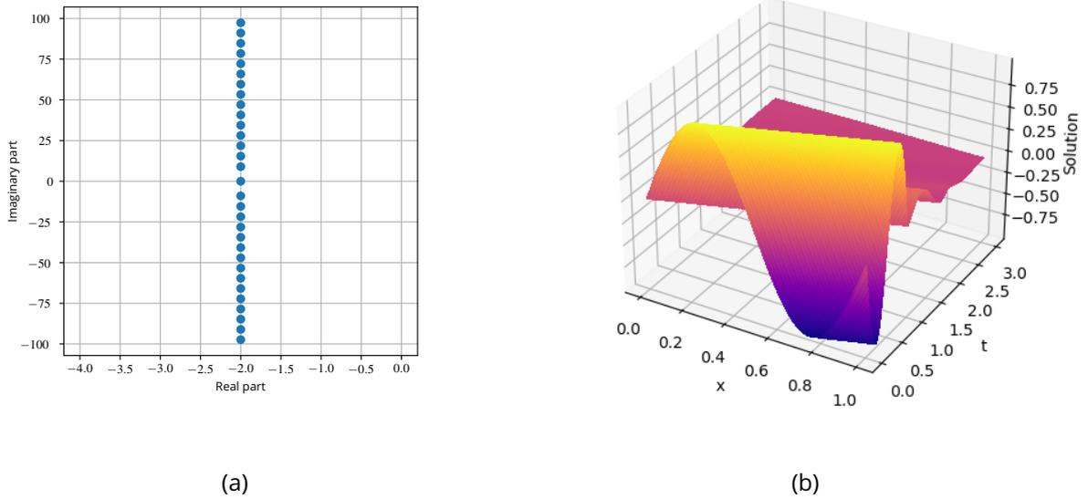
Figure 1: (a) Spectrum distribution of (4) and (b) solution of (2) with initial condition  $\varphi(0, x) = \sin(2\pi x)$ , with  $\frac{L}{\lambda} = 1$  and parameters  $k_p$  and  $k_i$  satisfying (5). Figure taken from [12].
