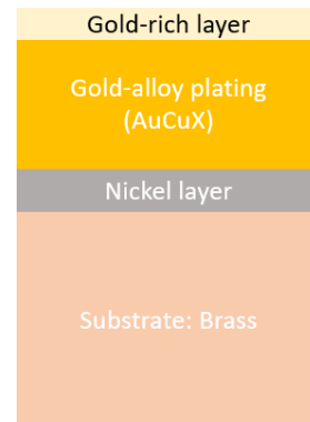
Fig. 4. Detail of the different layers composition of the disc coating (not to scale)
