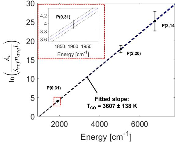
**Fig. 10** Multi-line Boltzmann regression of the CO features probed at 4.98  $\mu\text{m}$  in this study on a 1.09 Torr, 3.28 km/s shock at  $t = 5 \mu\text{s}$ . The temperature estimated from the slope is  $3607 \pm 138 \text{ K}$ .
