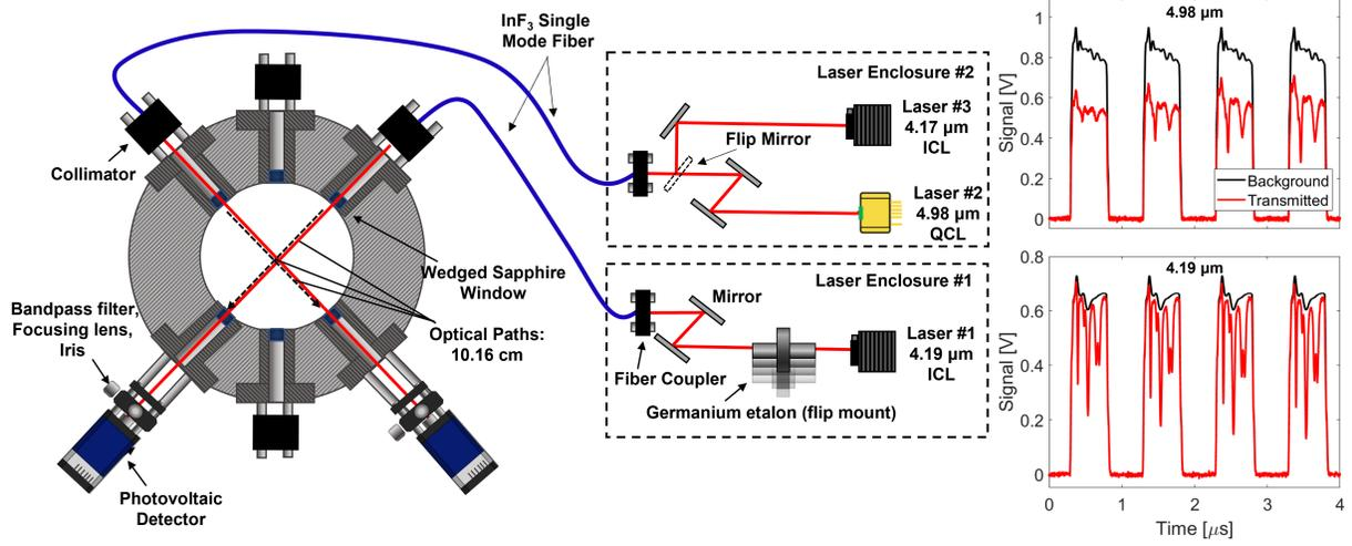
**Fig. 3** Optical setup on the EAST facility. Two laser enclosures contain the beam and couple the light into InF<sub>3</sub> single mode fibers. The 4.17- $\mu\text{m}$  ICL laser or the 4.98- $\mu\text{m}$  QCL laser were used depending on the expected shock speed (left). Representative background and transmitted light intensity signals for the first 4  $\mu\text{s}$  of a test (right).
