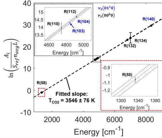
**Fig. 9** Multi-line Boltzmann regression of the CO<sub>2</sub> transitions probed in this study on a 1.99 Torr, 3.29 km/s shock at  $t = 5 \mu\text{s}$ . Note both the 4.19 and 4.17  $\mu\text{m}$  wavelengths are utilized as all 8 CO<sub>2</sub> features were well resolved on this test. The temperature estimated from the slope is  $3546 \pm 76 \text{ K}$ . Absorbance feature labels in black and blue denote  $\nu_3(00^0 0)$  and  $\nu_3(01^1 0)$  transitions respectively.
