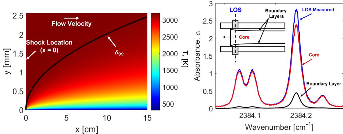
**Fig. 4** (left) Simulated compressible boundary layer temperature profile. The shock location,  $\delta_{99}$  thickness and freestream flow direction are highlighted. The no slip condition is enforced at the wall ( $y = 0$ ). (right) Absorbance signals from the line of sight (blue), core (red), and boundary layer (black) estimated from a similarity solution of the boundary layer profile.
