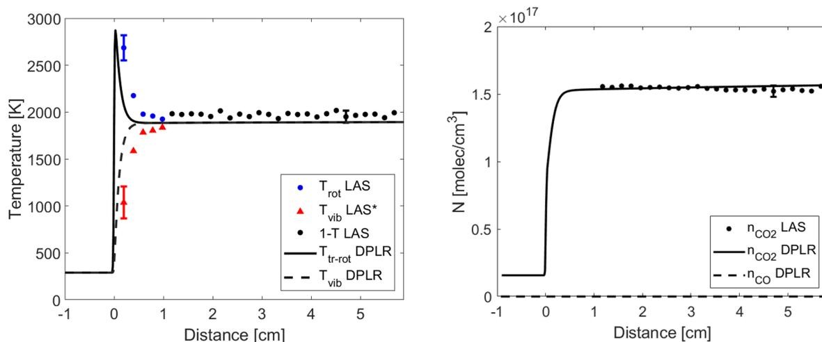
**Fig. 19** Time resolved rotational and vibrational temperature shown in blue and red (left) and number density (right) for a 1.96 km/s shock with 0.49 Torr fill pressure. The vibrational temperature is determined from conservation of enthalpy assuming  $T_{tr} = T_{rot}$ .
