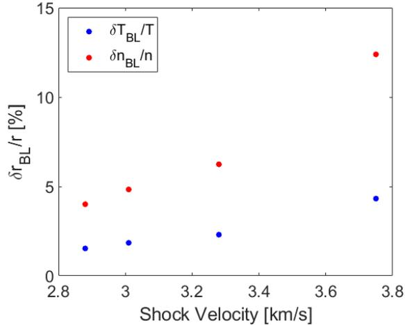
**Fig. 20 CO<sub>2</sub> temperature and number density uncertainty from the boundary layer assuming a  $\pm 10\%$  uncertainty to  $\delta_{99}$ .**
