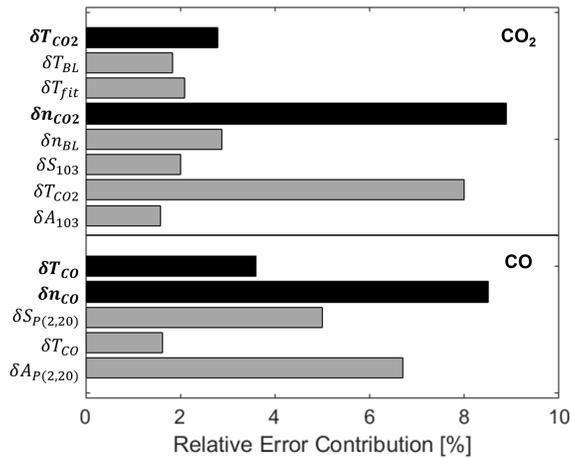
**Fig. 22** Bar chart representing the contribution of uncertainty of each term in Eq. 33 and 35 on a 3.01 km/s test case for CO<sub>2</sub> (top) and CO (bottom)
