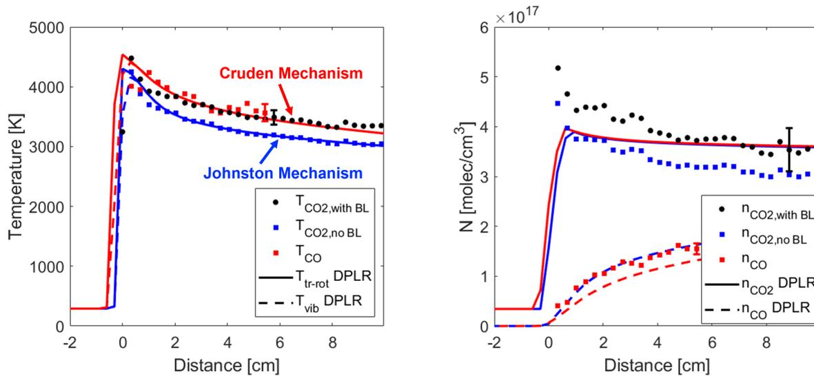
**Fig. 12** Temperature (left) and number density (right) vs distance behind shock estimated with (black) and without (blue) the boundary layer for a 3.40 km/s, 1.09 Torr fill pressure test case. CO data becomes optically thick halfway through the test.
