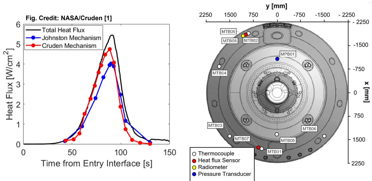
**Fig. 1** MEDLI2 flight data (total heat flux) compared to the radiative heat flux predicted by the Cruden [4, 5] and Johnston [6] mechanisms (left). Backshell measurement locations of the MEDLI2 sensor suite (right). Figure reproduced from [1–3, 7].
