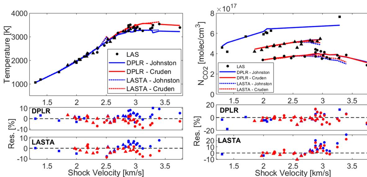
**Fig. 18** Measured temperature (left) and  $\text{CO}_2$  number density (right) vs shock velocity. Data is compared with the Cruden [4, 5] and Johnston [6] mechanisms simulated in DPLR [47] and the LASTA [42]+Cantera[48] model. Squares, triangles, and circles denote a fill pressure of 1.99, 1.49, and 1.09 Torr respectively.
