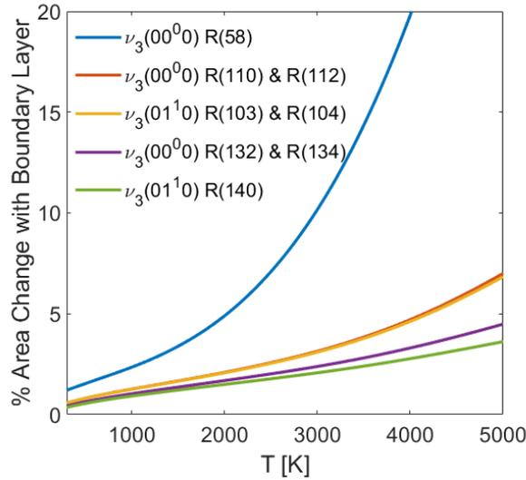
**Fig. 5 Sensitivity of path-integrated line intensity (measured absorbance area) to a representative simulated cold boundary layer ( $\approx 1$  mm) in the EAST facility assuming a similarity solution of a 2.96 km/s shock with a fill pressure of 1.49 Torr and scaled by variable core temperature (T).**
