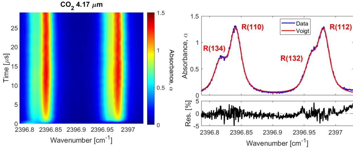
**Fig. 7** (left) Absorbance vs wavenumber and time for CO<sub>2</sub> spectrum at 4.17 μm. (right) Representative Voigt fit of spectrum at t = 11 μs.
