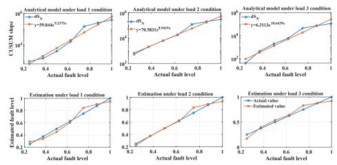
Fig. 11: Fault severity estimation
