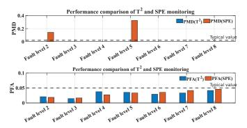
Fig. 8: Performance of NAP-based PCA fault detection
