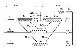
Fig. 3: Stator windings circuit under an inter-turn fault
