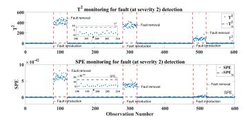
Fig. 7: Fault level 2 detection with NAP-based PCA
