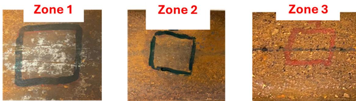
**Figure 4.** Various rail zones with different oxide thicknesses.
