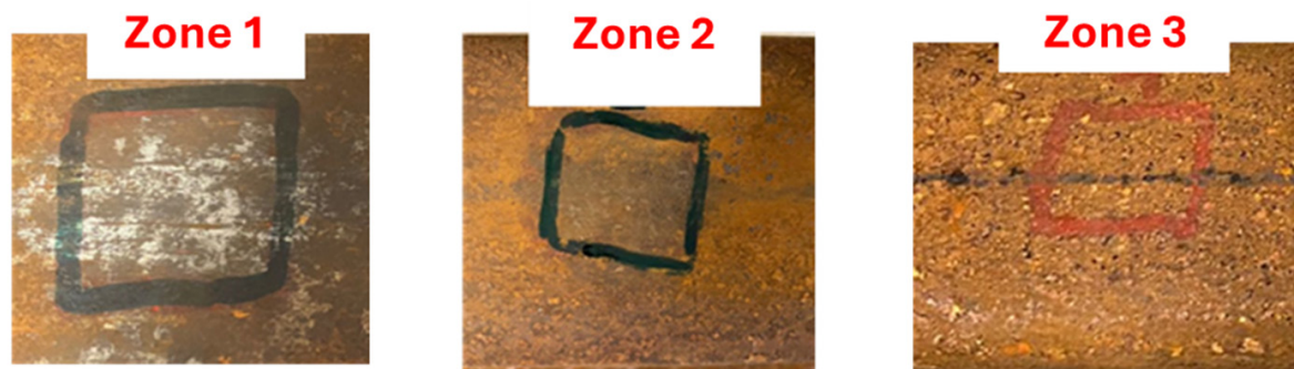
Figure 4. Various rail zones with different oxide thicknesses.
