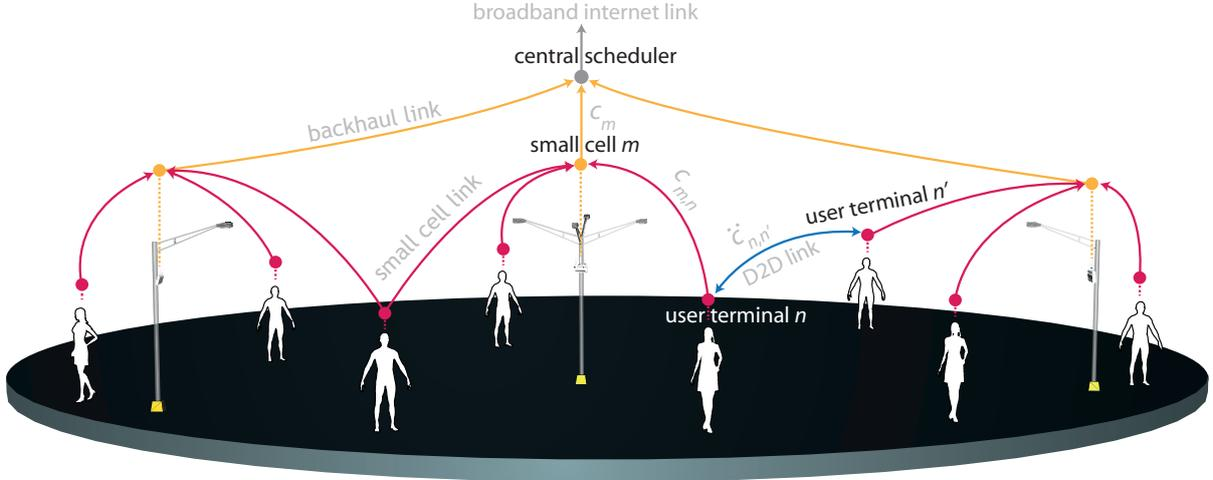
Figure 6.1: A sketch of the scenario given in the system model. A central scheduler is in charge of providing broadband connection to  $M$  SBSs via backhaul links. Depending on the users' contents availability in the caches of SBS and UTs, the SBSs serve their user either via wireless small cell links or D2D communications.
