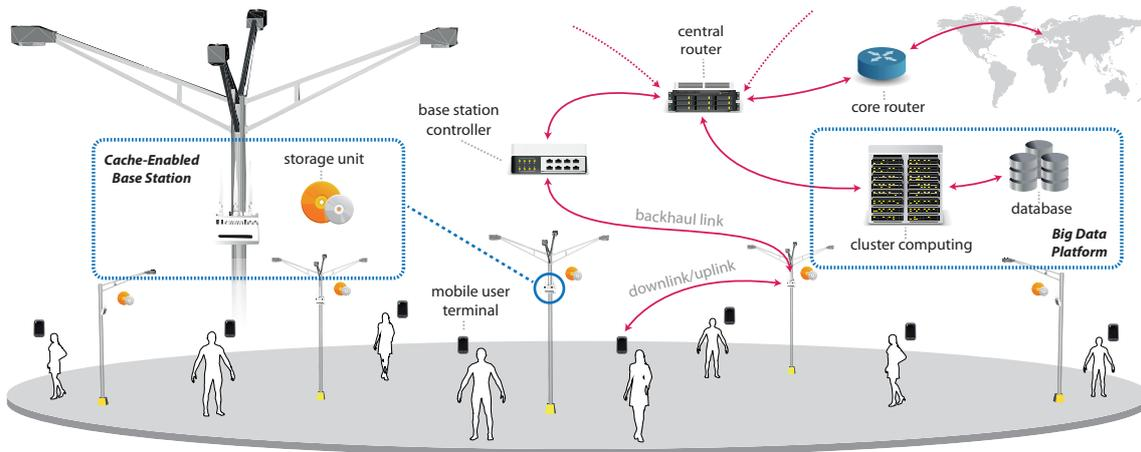
Figure 8.1: An illustration of the network model. A *big data platform* is in charge of tracking/predicting users' demand, whereas *cache-enabled base stations* store the strategic contents predicted on the big data platform.
