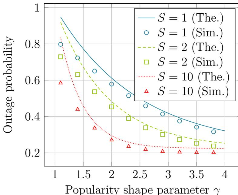
Figure 3.6: The evolution of outage probability with respect to the popularity shape parameter  $\gamma$ . SNR = 10 dB,  $\lambda = 0.2$ ,  $\gamma = 2$ ,  $L = 1$  nats,  $\alpha = 4$ ,  $C_1 = 0.0005$ ,  $C_2 = 0$ .
