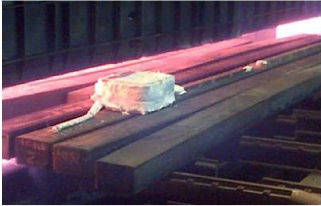
Figure 2.5: Instrumented bloom with thermal box before charging into the furnace
