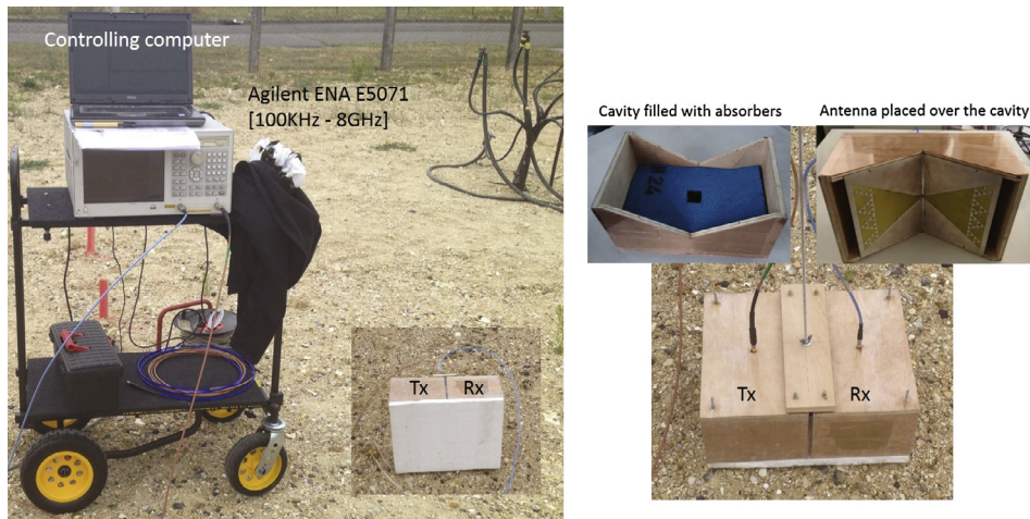
Fig. 13. (left) Vector Network Analyzer and controlling computer, (right) transmitting and receiving antennas cavity backed V-folded bowtie antennas.
