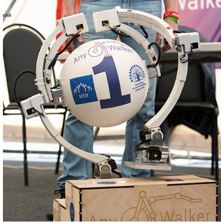
Figure 2.2: AnyWalker robot uses reaction wheels as an auxiliary stabilization system; see [28, 29].
